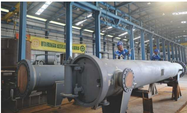
Pig launcher & Receiver – Jambaran Tiung Biru Tiung Biru Gas Development Project PT Pertamina EP Cepu
