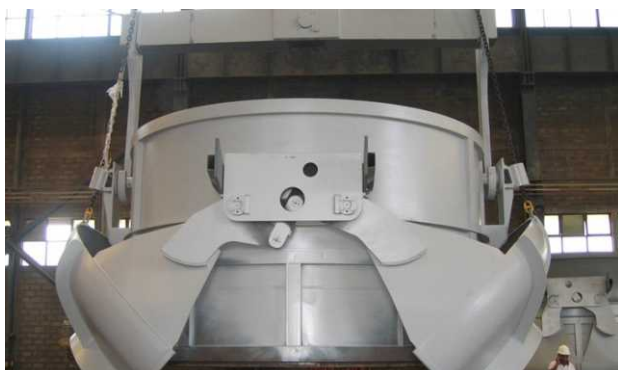
Scrap Charging Bucket PT. Ispatindo Surabaya
