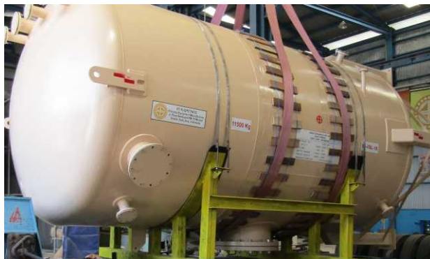
Loaded Carbon Vessel – Oxide Expansion PT Bumi Suksesindo
